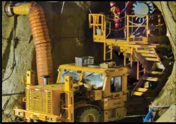
Designed to provide a safe work platform for installation of services in tunnel headings up to six meters (20 feet) high. The Mine-Mate™ SL2 & SL3 Scissor Lifts are fully equipped as standard for the multi-tasking required in today's underground trackless mining environment. The SL3 is available with an industry-first 3600Kg deck capacity and attachment system.
